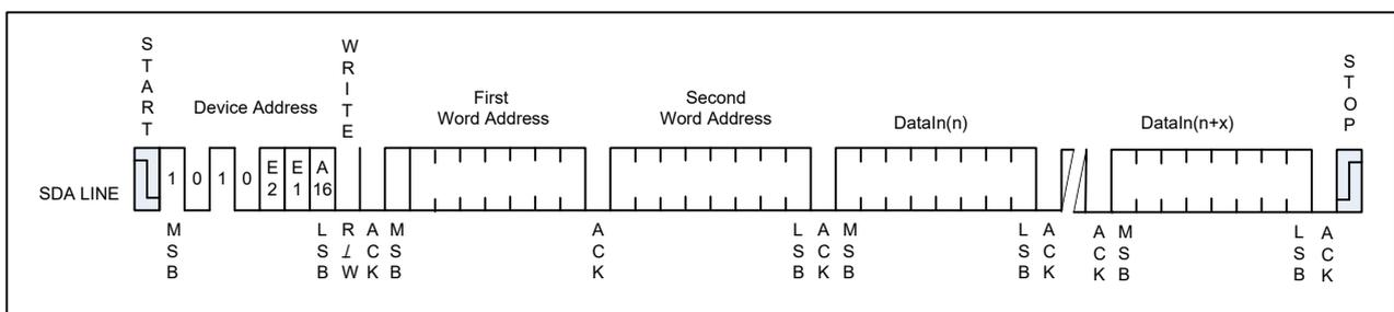
The lower eight bits of the data word address are internally incremented following the receipt of each data word. The higher data word address bits are not incremented, retaining the memory page row location. When the word address, internally generated, reaches the page boundary, the following byte is placed at the beginning of the same page. If more than 256 data words are transmitted to the P24CM01H, the data word
