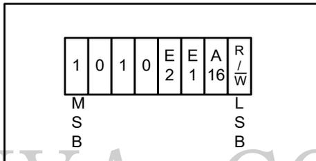
The two E2 and E1 device address bits allow as many as four devices on the same bus. These bits must compare to their corresponding hardwired input pins.
