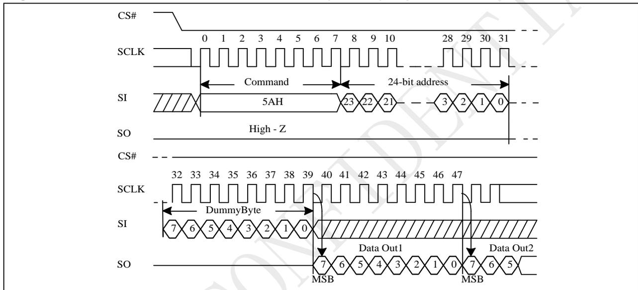
Figure 10-44 Serial Flash Discoverable Parameter (SFDP) Table
