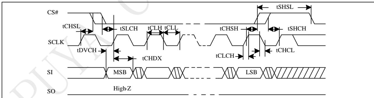
Figure 5-5 Output Timing
