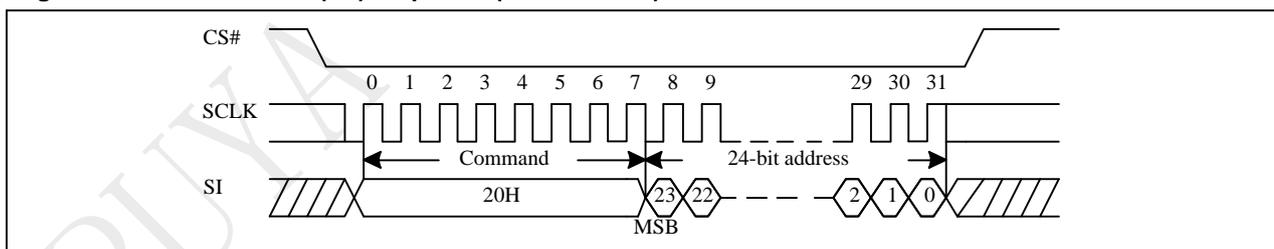
The self-timed Sector Erase Cycle time ( $t_{SE}$ ) is initiated as soon as Chip Select (CS#) goes high. The Write in progress (WIP) bit still can be check out during the Sector Erase cycle is in progress. The WIP sets 1 during the  $t_{SE}$  timing, and sets 0 when Sector Erase Cycle is completed, and the Write Enable Latch (WEL) bit is reset. If the sector is protected by BP4, BP3, BP2, BP1, BP0 bits, the Sector Erase (SE) instruction will not be executed on the sector.
