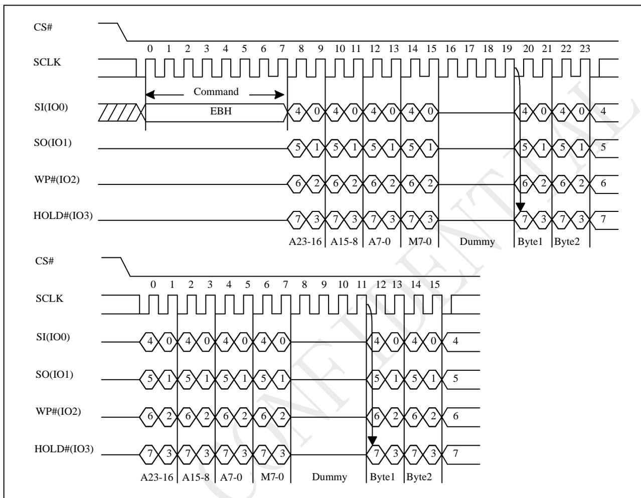
Note: 1. 4 X IO Read Performance Enhance Mode, if M5-4 = 1, 0. If not using performance enhance recommend to set M5-4 ≠ 1, 0.
