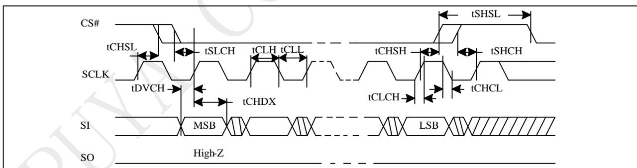
Figure 5-5 Output Timing
