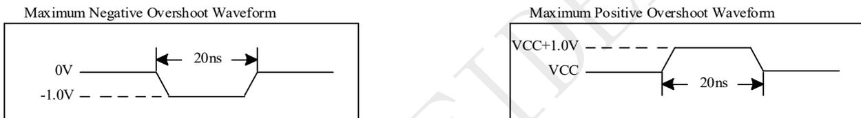
**Figure 5-2 Input Test Waveforms and Measurement Level**
