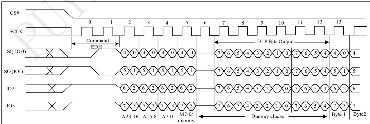
**Figure 9-23n DTR Burst Read with Wrap with DLP bits output Sequence**
