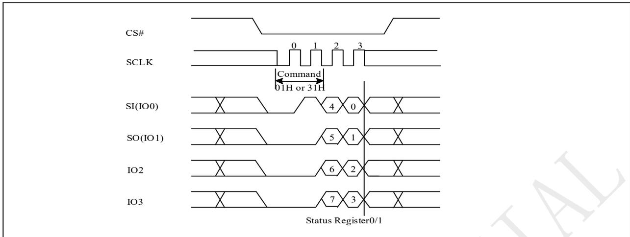
**Figure 9-7b Write Status Register (WRSR) Sequence (Command 01, 2 bytes' data)**
