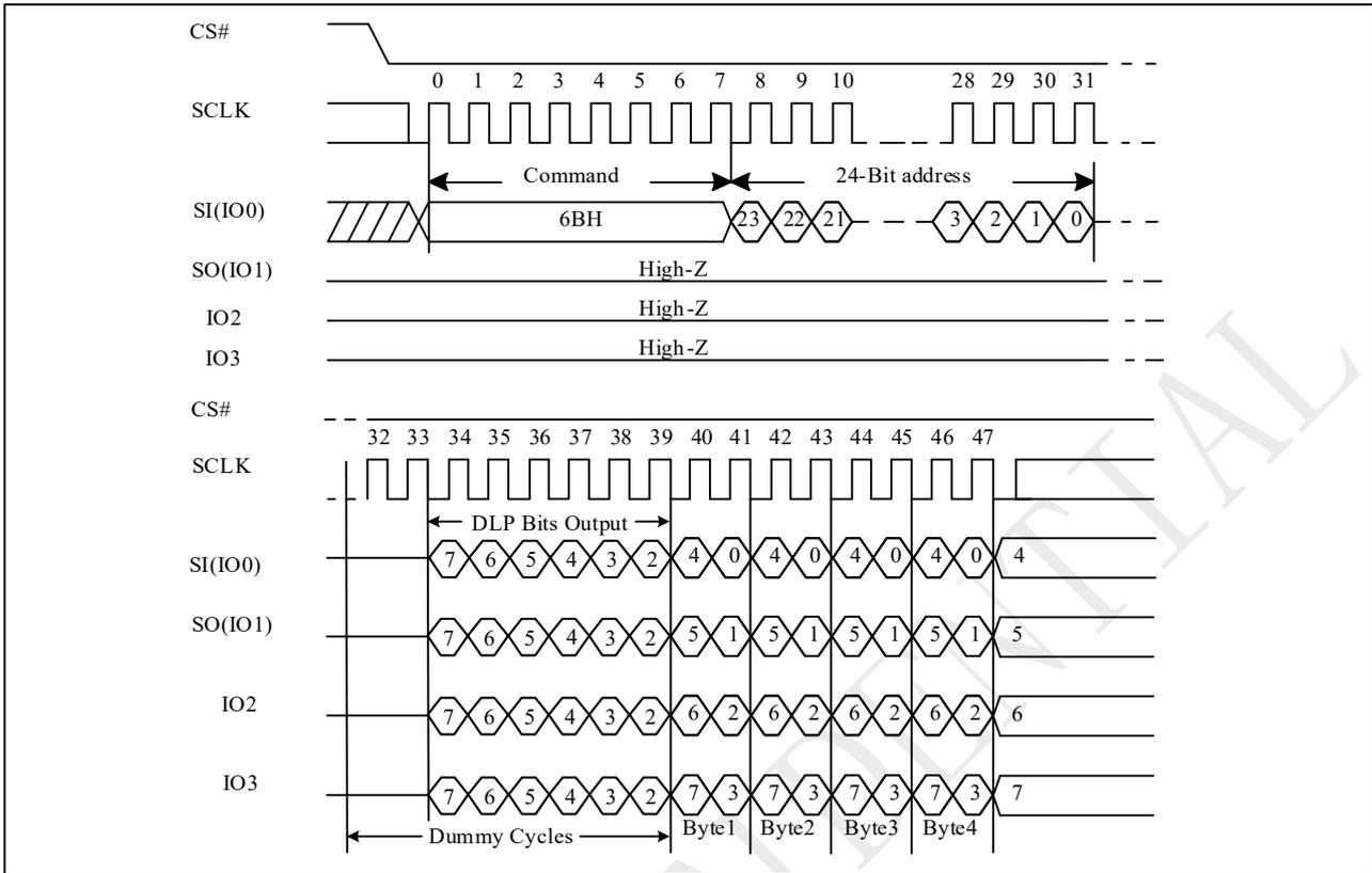
Figure 9-23e 4IO Read with DLP bits output Sequence
