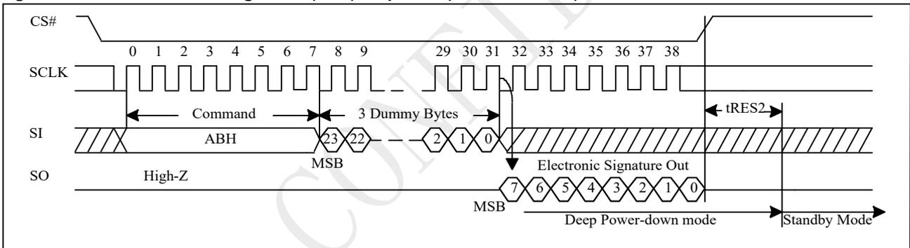
**Figure 9-36a Read Electronic Signature (RES) Sequence (QPI)**
