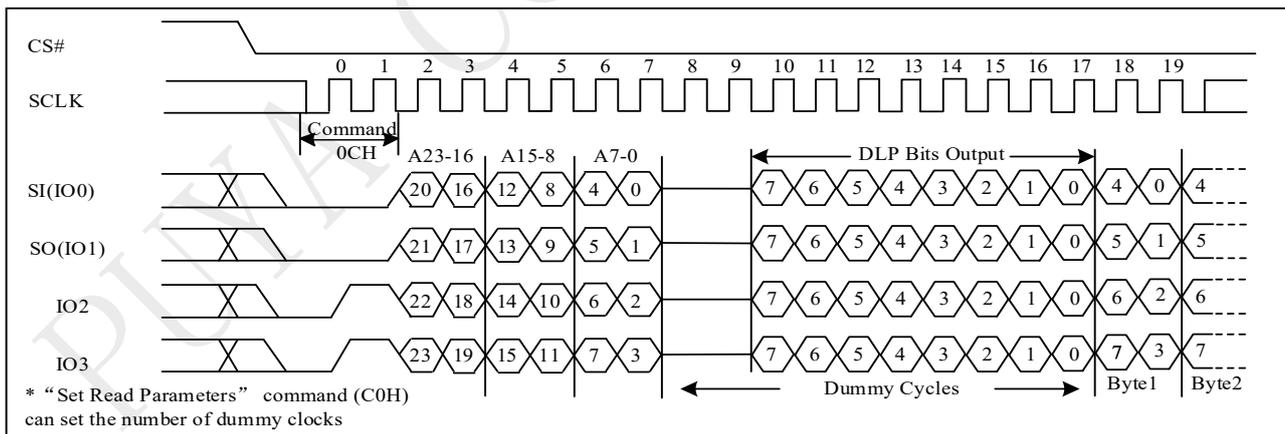
Figure 9-23i DTR Fast Read with DLP bits output Sequence
