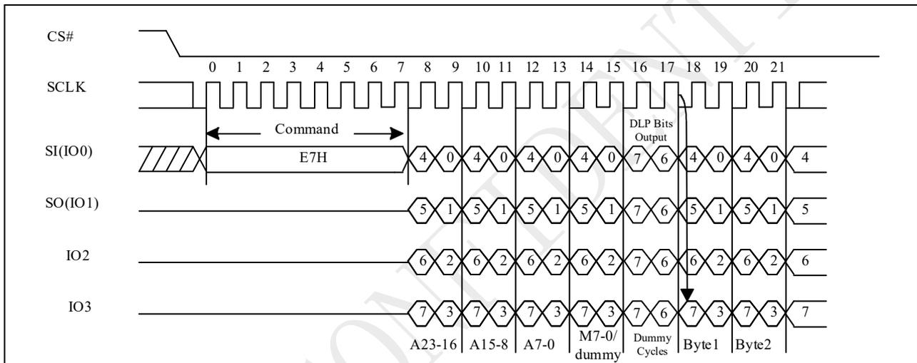
**Figure 9-23h Burst Read with Wrap with DLP bits output Sequence**
