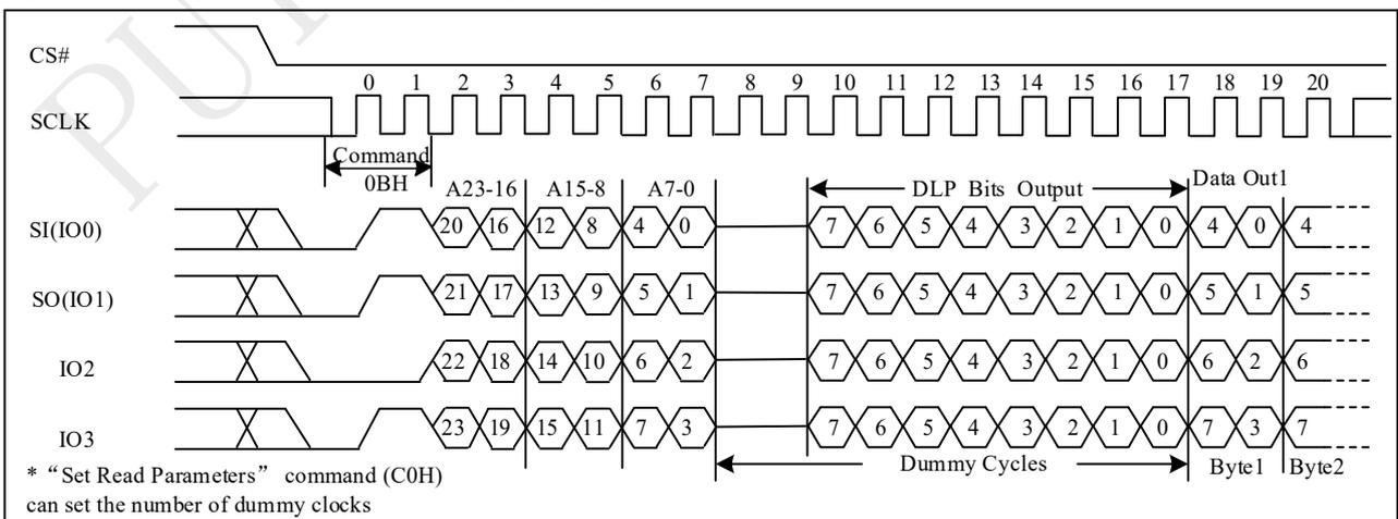
**Figure 9-23b Dual Read with DLP bits output Sequence**
