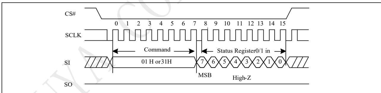
**Figure 9-7a Write Status Register (WRSR) Sequence (QPI)**
