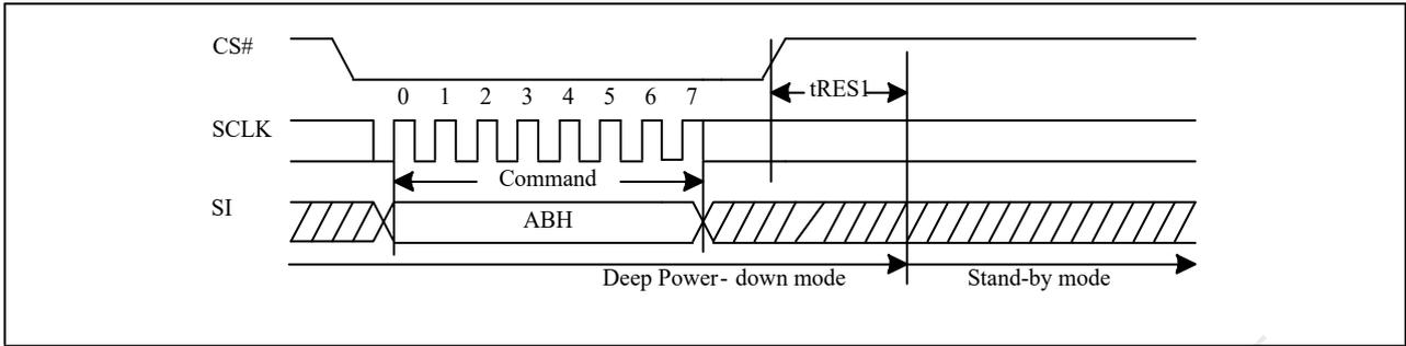
**Figure 9-36c Release from Deep Power-down (RDP) Sequence (QPI)**
