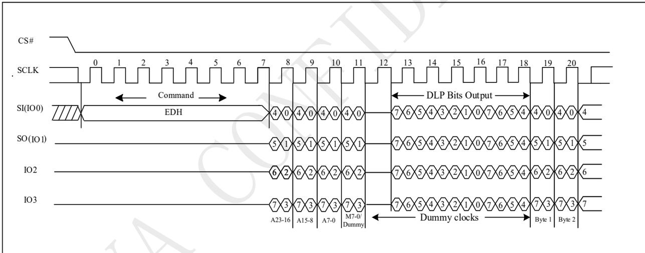
**Figure 9-23m DTR 4IO Read with DLP bits output Sequence in QPI mode**
