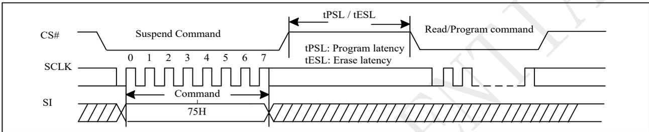
**Figure 9-42a Suspend to Read/Program Latency (QPI)**
