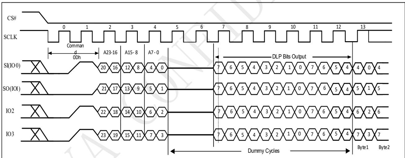
**Figure 9-23k DTR 2IO Read with DLP bits output Sequence**
