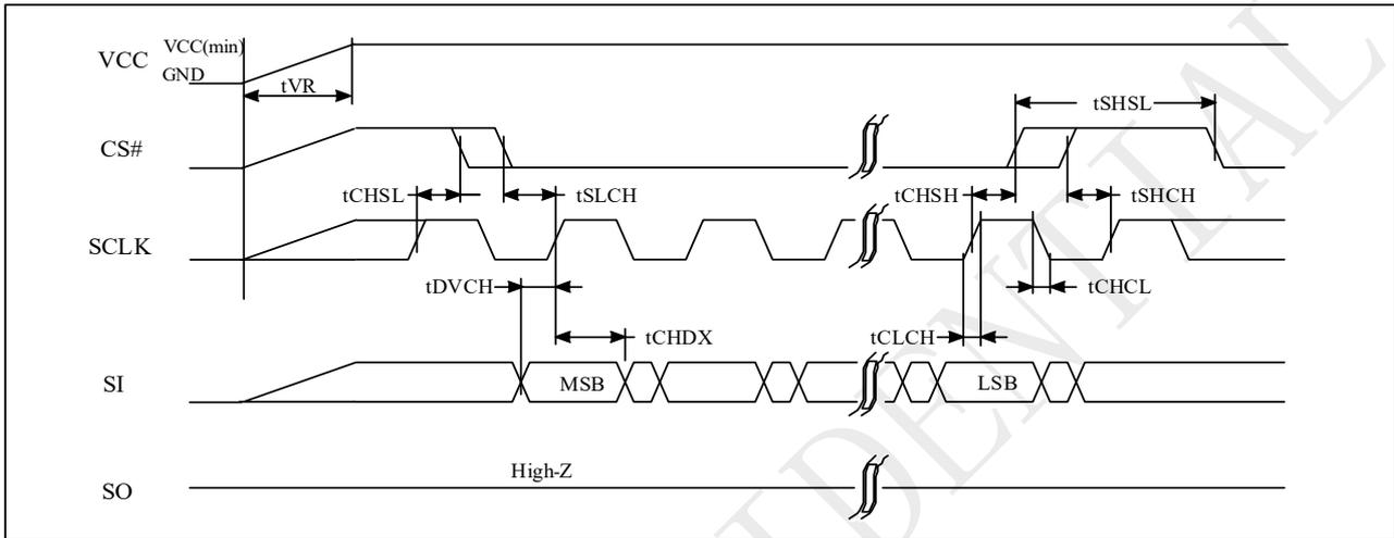
**Figure 5-9 Power-Up Timing**
