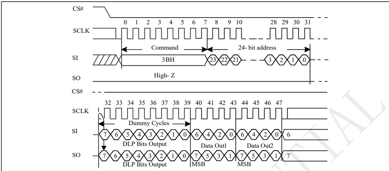
**Figure 9-23c 2IO Read with DLP bits output Sequence**
