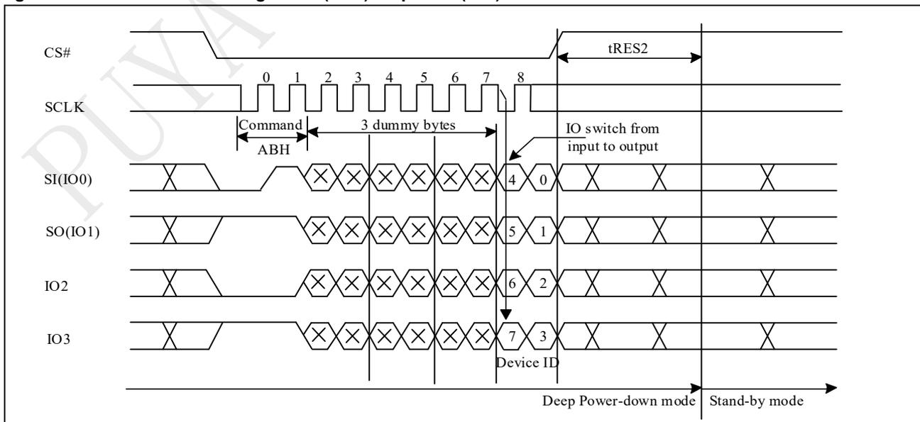
**Figure 9-36b Release from Deep Power-down (RDP) Sequence (Command ABh)**
