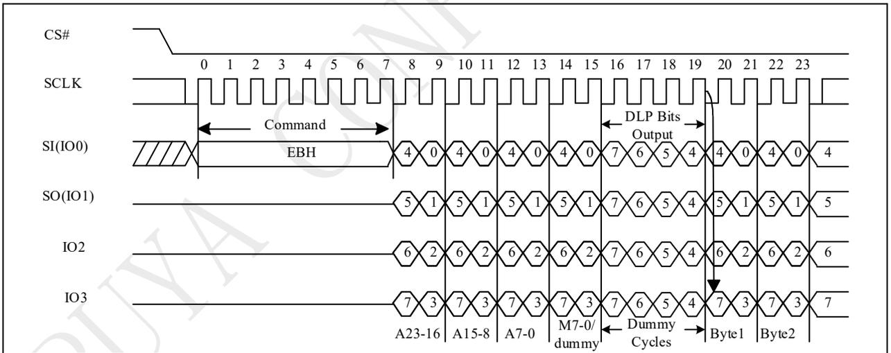
**Figure 9-23f 4IO Read with DLP bits output Sequence in QPI mode**
