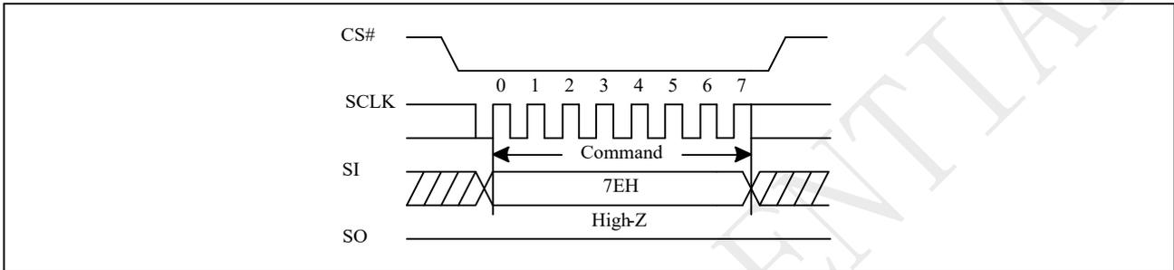
**Figure 9-48a Global Block Lock (QPI)**
