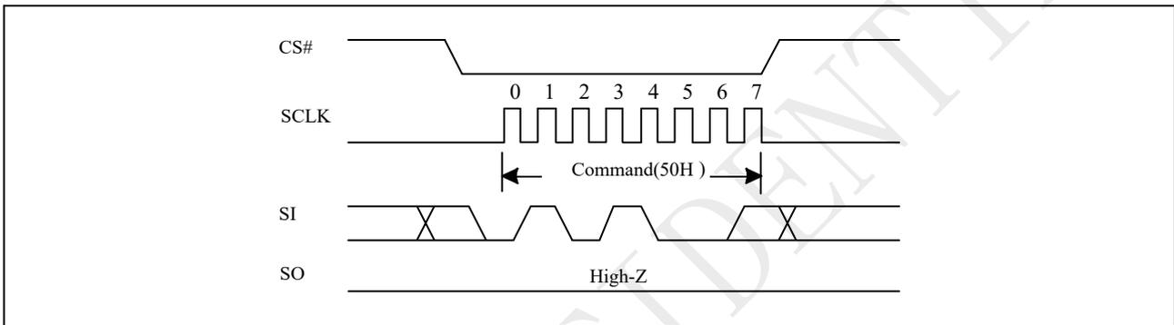
**Figure 9-4a Write Enable for Volatile Register Sequence (QPI)**
