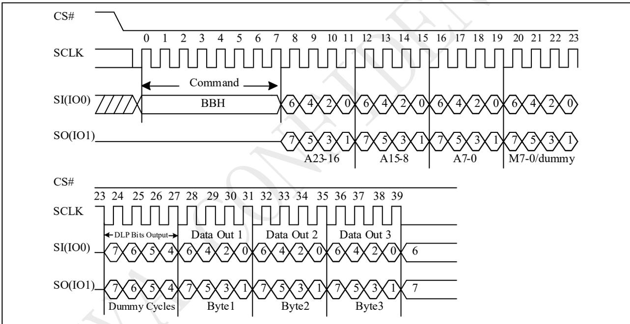
Figure 9-23d Quad Read with DLP bits output Sequence
