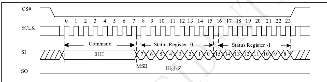
**Figure 9-7c Write Status Register (WRSR) Sequence (QPI)**
