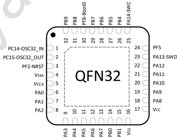
图 3-5 QFN32(4\*4) PY32F040K3xU7-E Pinout3 (Top view)
