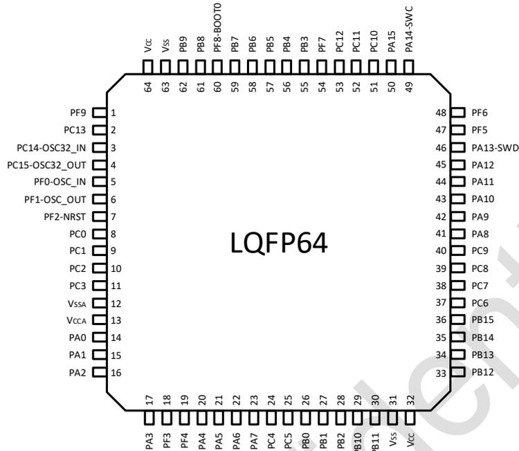
图 3-1 LQFP64 PY32F040R1xT7-E Pinout1 (Top view)
