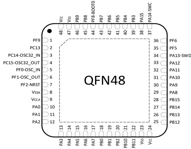
图 3-3 QFN48 PY32F040C1xU7-E Pinout1 (Top view)
