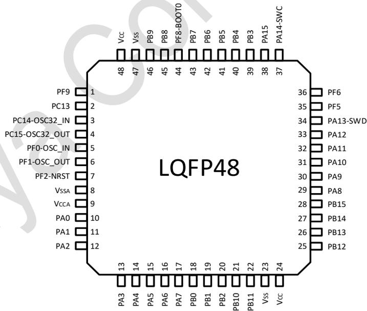
图 3-2 LQFP48 PY32F040C1xT7-E Pinout1 (Top view)
